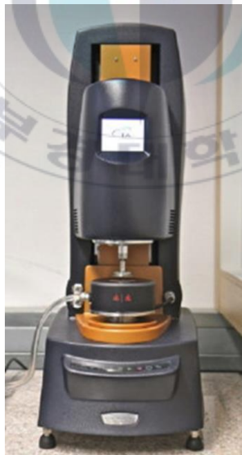
Figure 14. The experimental setup of HR-2 TA Instruments rheometer.
