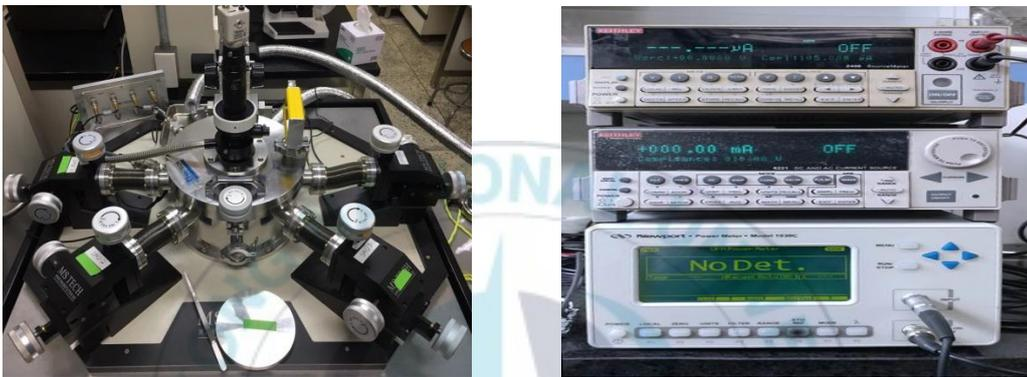
**Figure 11.** Vacuum probe station in our lab and Kethley Source-Measure Unit
