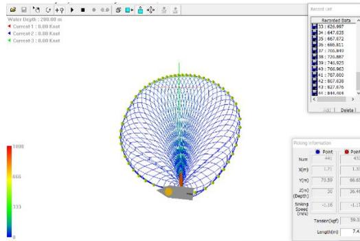
Figure 15. Shapes of the tuna purse seine with no current from shooting to hauling in process.
