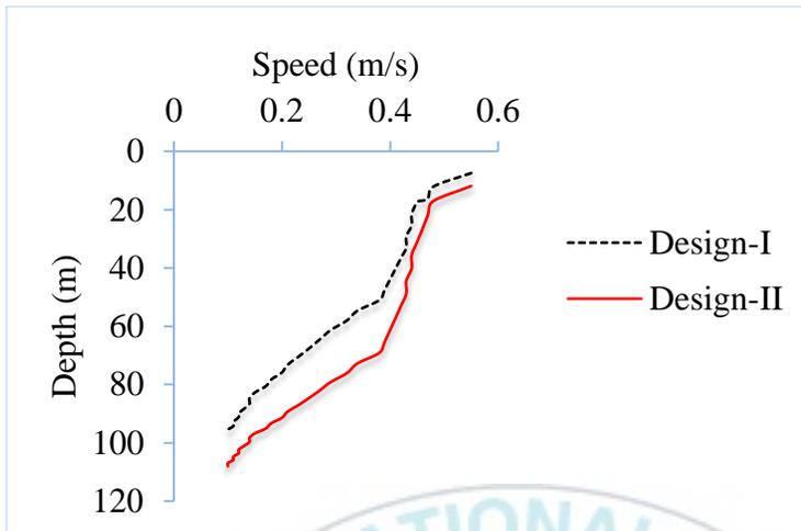
Figure 20. Sinkers line weight speed by depth of the two Design gears.
