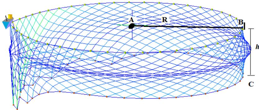
Figure 10: Schematic diagram for computation of surrounding volume of the purse seine gear. Source (Author).
