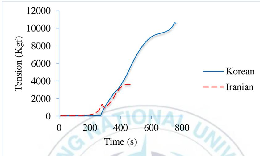
Figure 13. Tension on the ring lines of the tuna purse seine with no current.
