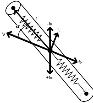
Figure 9. The mass-spring model illustrating the vector notation of the mesh bar. Source: (Lee, et al., 2007).
