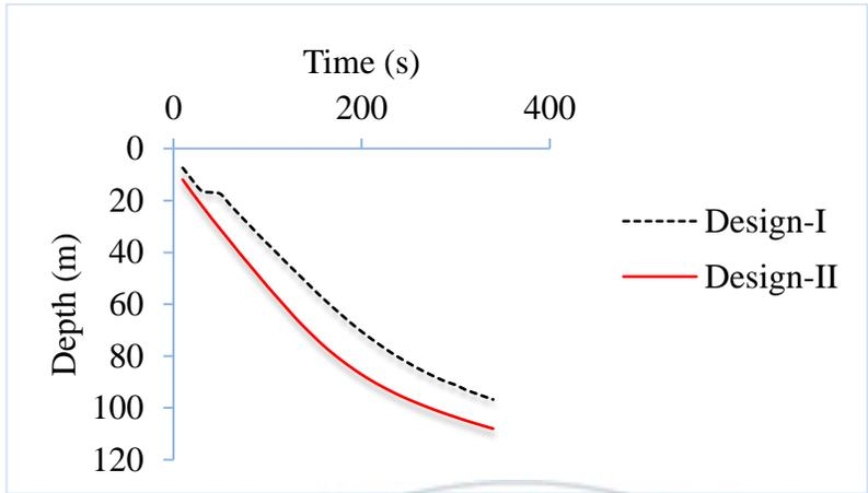
Figure 18. Sinking depth of the leadlines Design-I enlarged and deepened, and Design-II rigged with same weight as the Korean.
