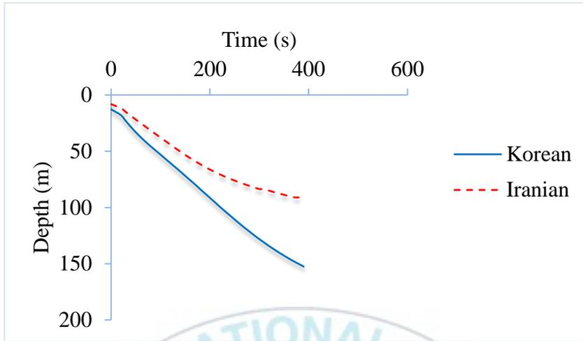
Figure 11. Sinking depths of the leadlines of tuna purse seine gears.
