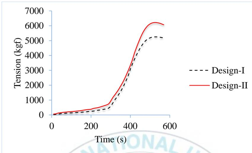
Figure 21. Tension on the purse line of the two Design gears.
