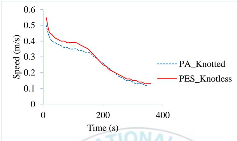
Figure 24. Sinking speed performance of the modified netting material (Design-III).
