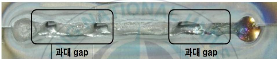
Fig. 1.2 Gap bridging failure due to excessive gap in lap joint fillet welding<sup>2)</sup>
