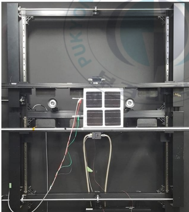
Figure 27. Solar simulator used to measure 2 × 2 module efficiency by courtesy of the photovoltaic laboratory, Korea Institute of Energy Research
