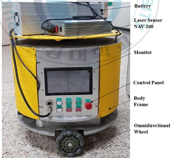
Fig. 2.1 OAGV system used for the thesis
