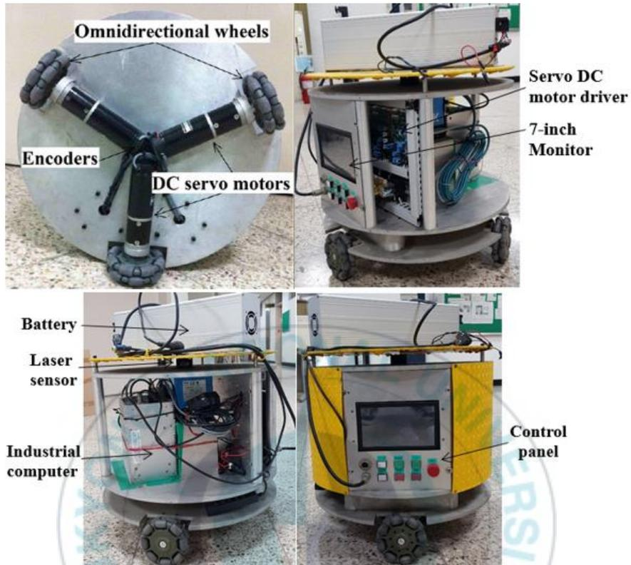
Fig. 2.2 Structure of the OAGV used for experiment
