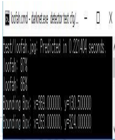
(a) Detected bounding box of loofah (b) Results of the bounding box
