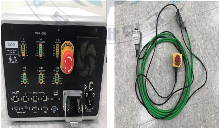
Fig. 2.2.5 Motor driver, cable for connect manipulator, and emergency stop button
