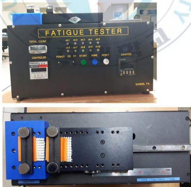
Fig 26. Stretching test machine
