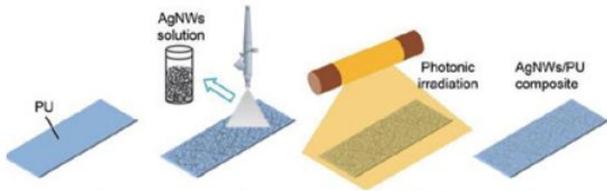
Fig 12. Schematic representation shows the fabrication steps of AgNWs/PU electrode.
