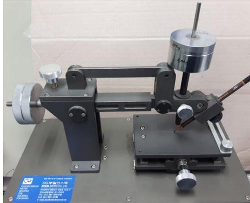
Fig 24. Pencil hardness tester
