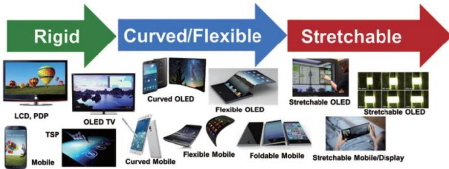
Fig 5. Rigid, flexible, and stretchable displays based on glass substrate, flexible substrate and stretchable substrates.
