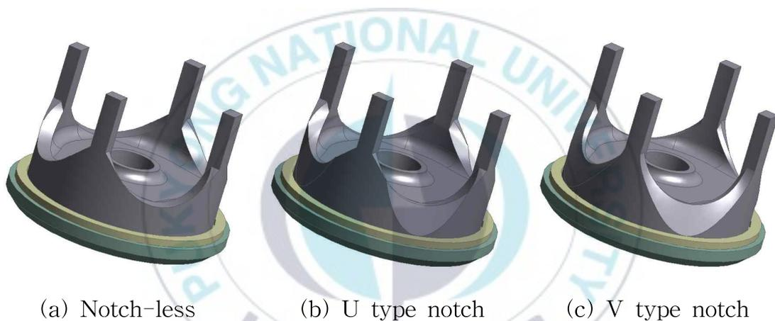
Fig. 3-1 3-type cone shape of designed globe valve
