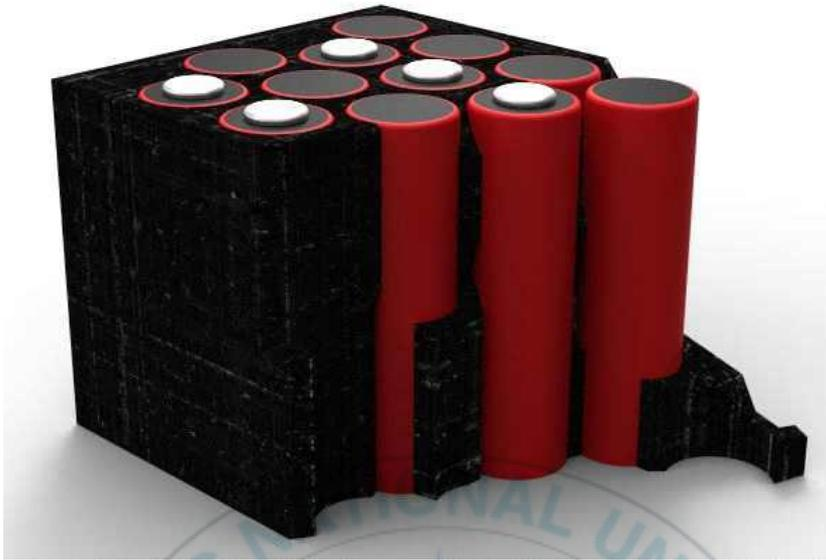
Fig. 1.4 Battery Module with PCM/graphite thermal management
