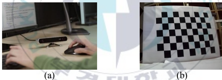
Fig. 5.1 Camera calibration setup (a), and image pattern for calibrating intrinsic parameter (b)
