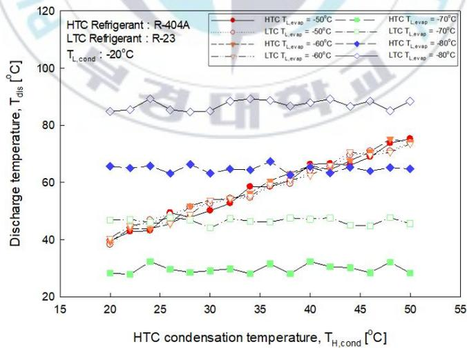
Fig. 3.5 Discharge temperature of HTC, LTC according to HTC condensation temperature
