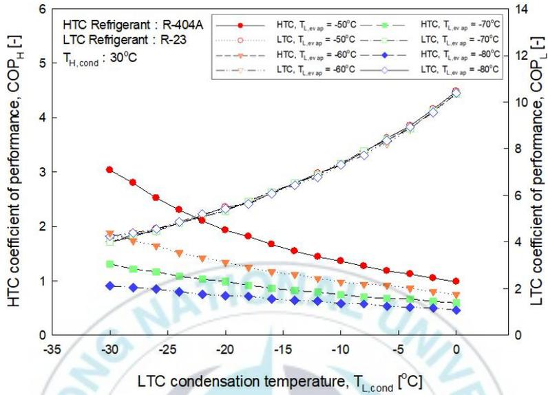
Fig. 3.20 COP of HTC, LTC according to LTC condensation temperature
