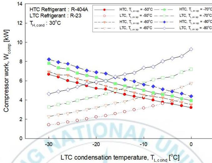
Fig. 3.18 Power consumption of HTC, LTC compressor according to LTC condensation temperature
