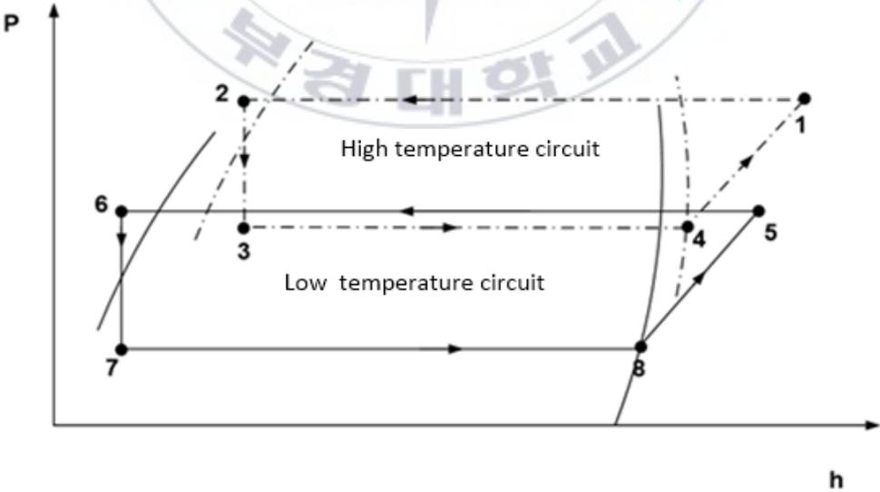
Fig. 1.2 Pressure-enthalpy diagram of cascade refrigeration system
