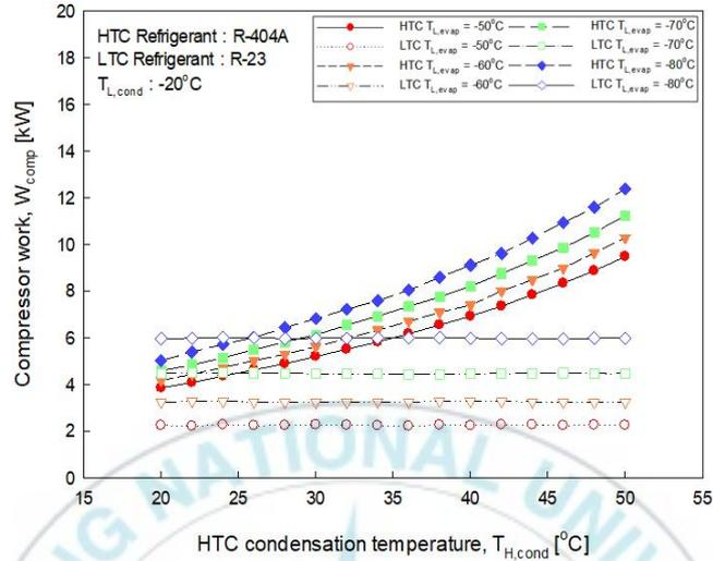
Fig. 3.4 Power consumption of HTC, LTC compressor according to HTC condensation temperature
