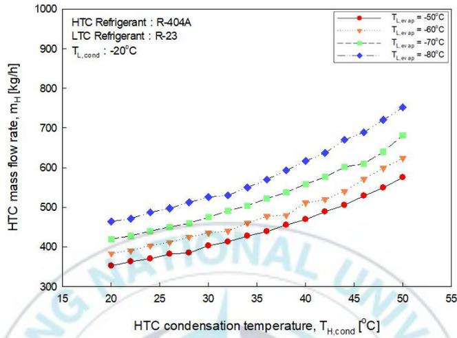
Fig. 3.1 Refrigerant mass flow rate of HTC according to HTC condensation temperature
