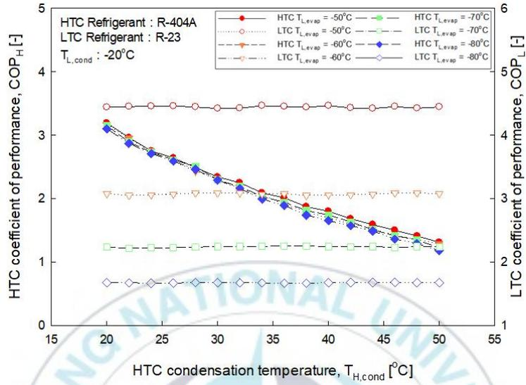
Fig. 3.6 COP of HTC, LTC according to HTC condensation temperature
