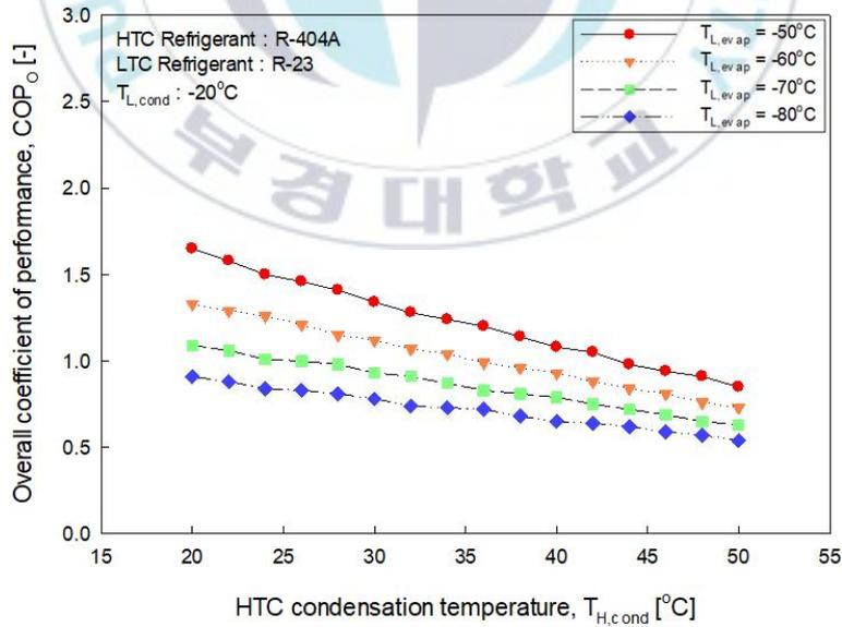
Fig. 3.7 Overall COP according to HTC condensation temperature
