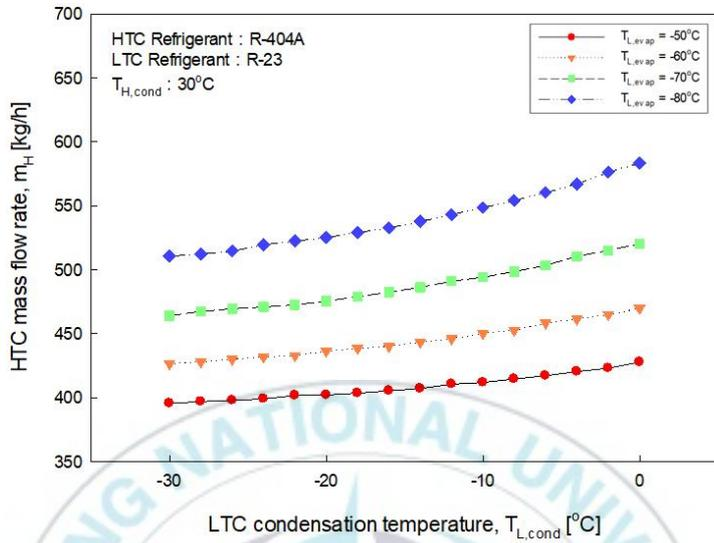
Fig. 3.15 Refrigerant mass flow rate of HTC according to LTC condensation temperature
