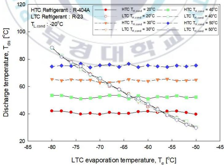
Fig. 3.12 Discharge temperature of HTC, LTC according to LTC evaporation temperature
