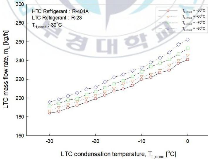
Fig. 3.16 Refrigerant mass flow rate of LTC according to LTC condensation temperature
