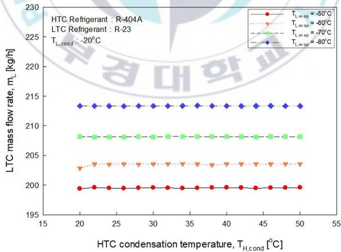
Fig. 3.2 Refrigerant mass flow rate of LTC according to HTC condensation temperature
