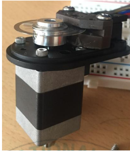
Figure 9: Stepper motor is attached with an encoder
