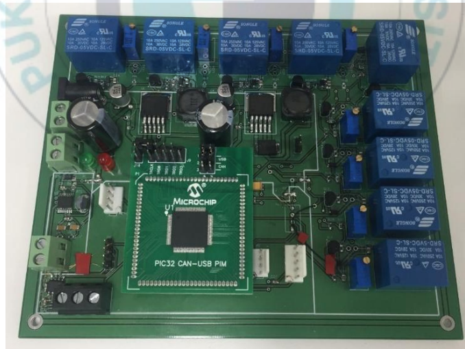
Figure 37: Controller PCB after soldering all components
