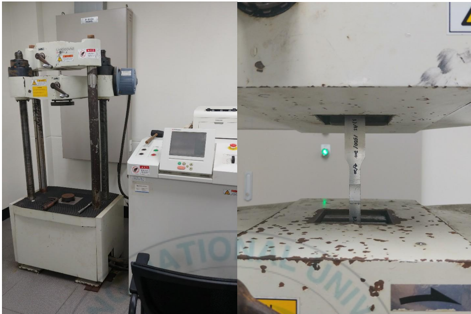
Fig. 4.2 Tensile strength test machine
