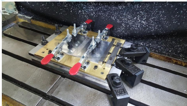
Fig. 3.2 Exclusive use jig of FSW
