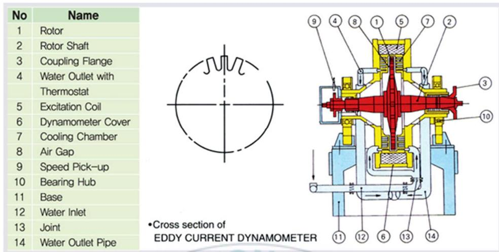
Figure 3. 2 Cross-section of the dynamometer
