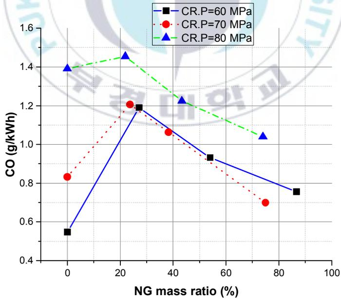
Figure 4. 7 CO emissions at 23.0 kW
