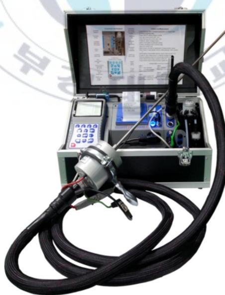
Figure 3. 4 Exhaust gas analyzer
