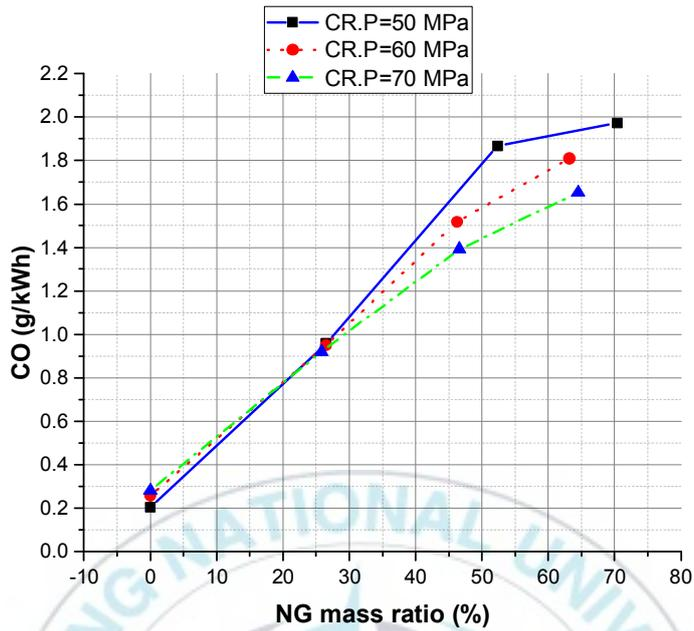
Figure 4. 6 CO emissions at 11.7 kW
