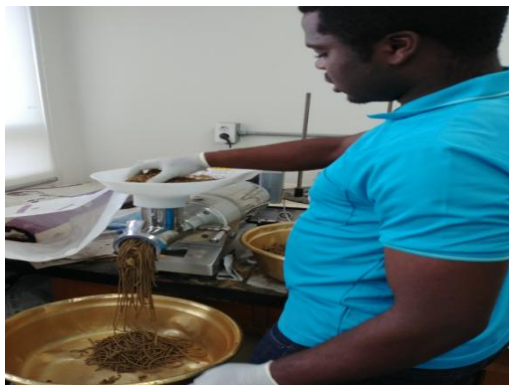
Fig. 4. Fish feed pelleting
