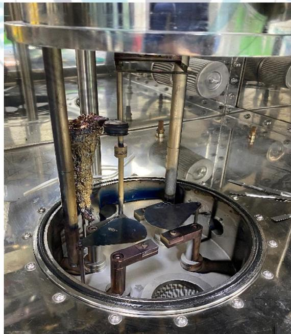
**Figure 18.** Thermal evaporator in my lab
