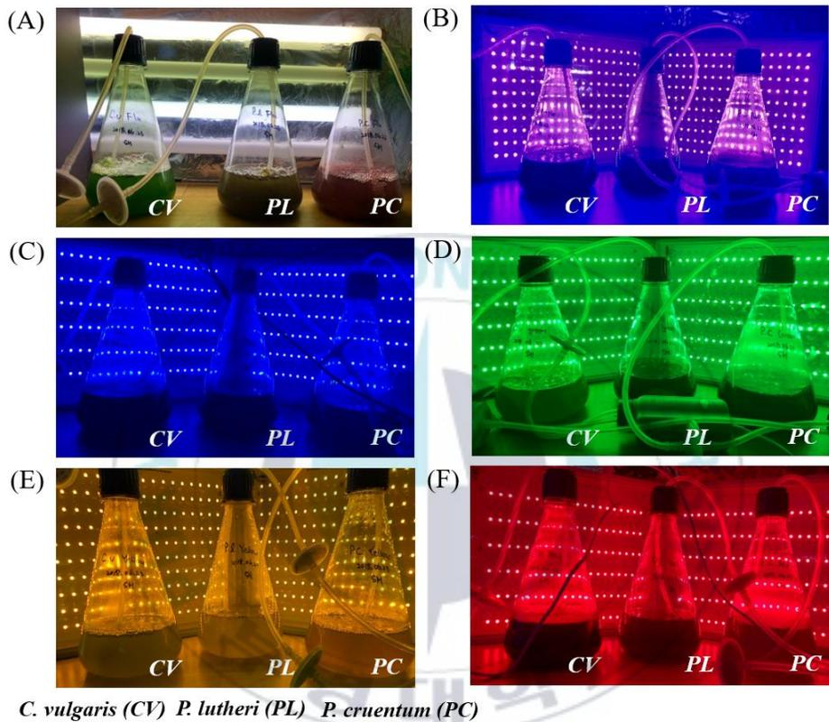
Figure 1. Photographs of microalgae cultured under different wavelengths; *C. vulgaris* (CV), *P. lutheri* (PL), and *P. cruentum* (PC), respectively. Cell culture was carried out under (A) fluorescent light as a control, (B) purple (400 nm), (C) blue (465 nm), (D) green (520 nm), (E) yellow (590 nm), and (F) red (625 nm) LED wavelengths.
