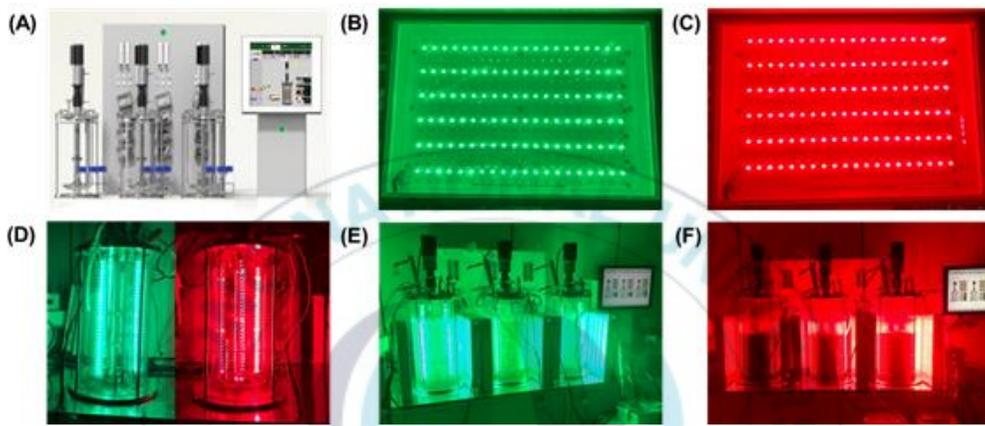
Figure 1. Application of three 14-L LED bioreactors. (A) Graphical photographs of the 14-L LED bioreactors. Photographs of the microalgae grown with external (B) green (520 nm) and (C) red LED (625 nm) panels and (D) internal LED light during the (E) first phase under the green LED wavelength for biomass culture and the (F) second phase under the red LED wavelength for lipid accumulation
