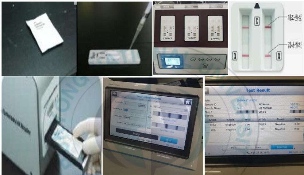
Fig. 13. Experimental procedure using the smart antibiotic residues system.
