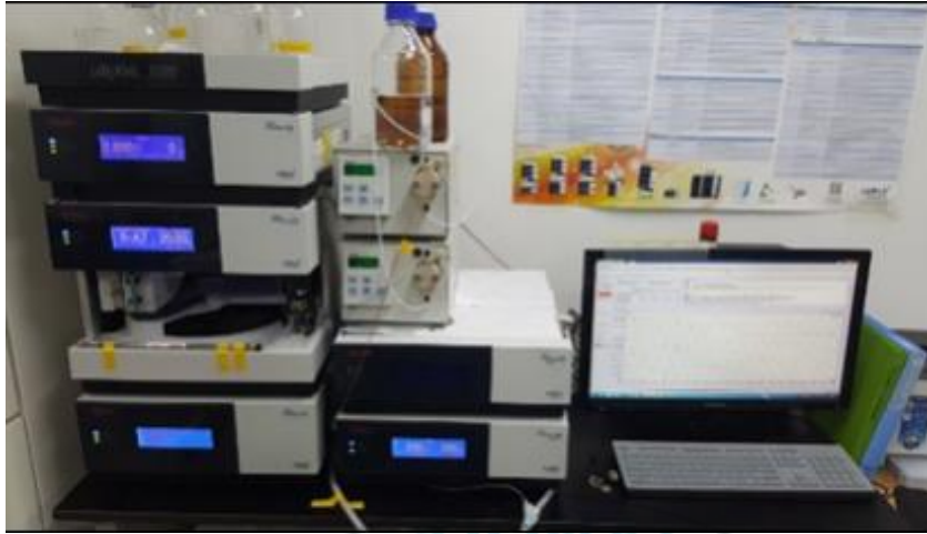
Fig. 4. High performance liquid chromatography using post-column oxidation method(AOAC, 2011) for paralytic shellfish poisoning (PSP) analysis.
