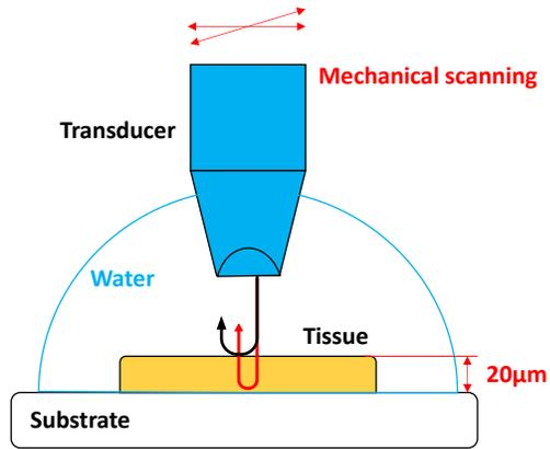
Figure 13 Demonstrate the schematic of tissue characterization by scanning acoustic microscope
