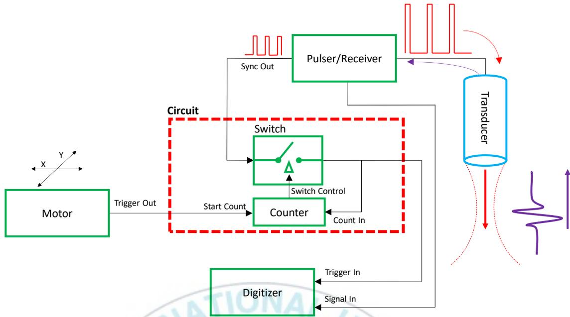
Figure 29 Demonstrate the diagram of synchronization of internal and external trigger
