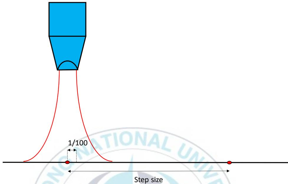
Figure 28 Demonstrate the distance to finish acquiring ten data in comparison with step size
