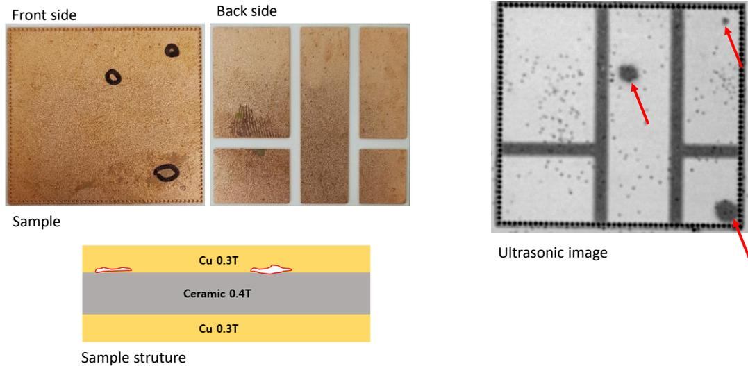
Figure 5 Demonstrates ultrasonic image of a multi-layers structure with air gaps stuck inside
