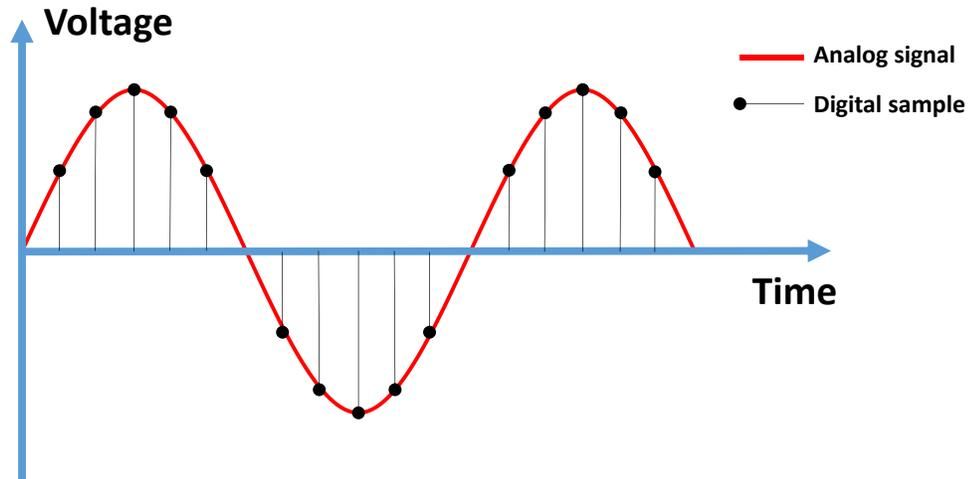
Figure 7 Demonstrate an analog signal after digital converter
