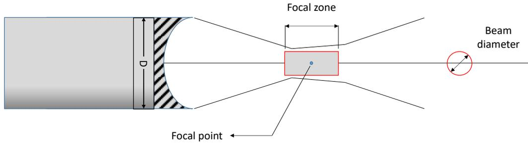
Figure 3 Beam profile of a single-element spherical transducer
