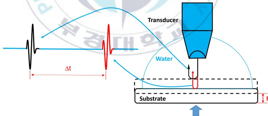
Figure 23 Demonstrate the diagram of acoustic speed measurement
