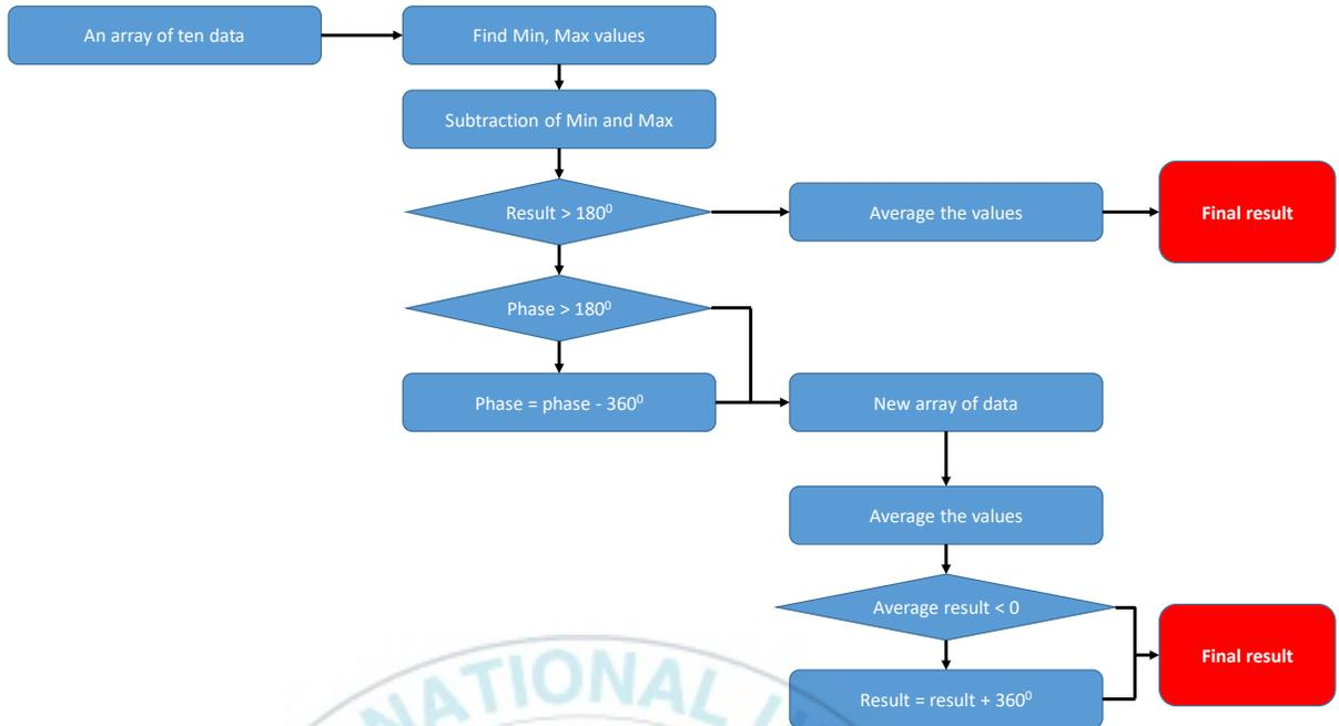
Figure 34 A flow chart for fixing error of average result due to phases distributed around zero
