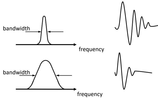
Figure 1 Demonstrate the relationship between waveform duration and bandwidth
