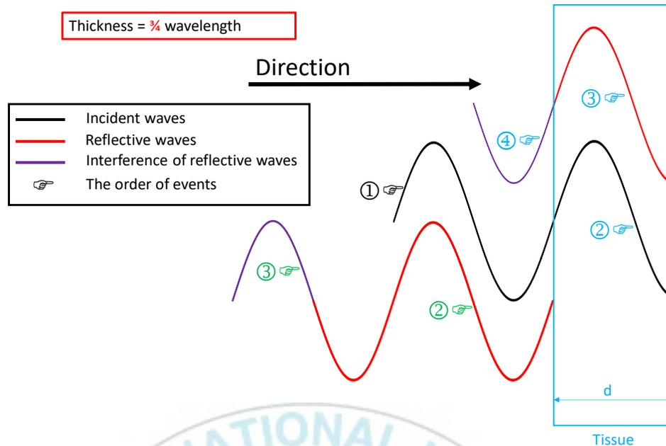
Figure 16 Demonstrate the case of thickness according to three fourth of wavelength
