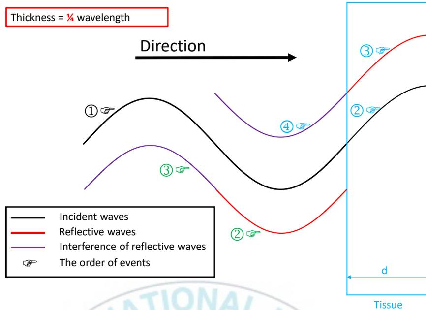
Figure 15 Demonstrate the case of thickness according to a quarter wavelength
