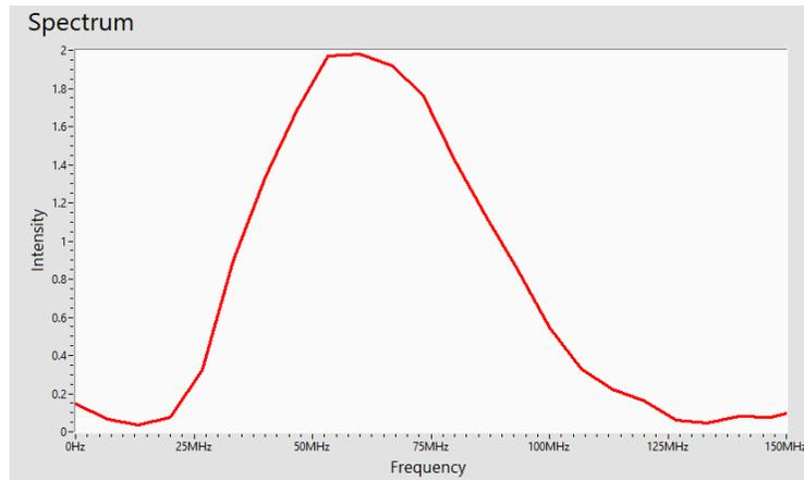
Figure 17 Indicate spectrum of the transducer with its signal reflected from glass surface
