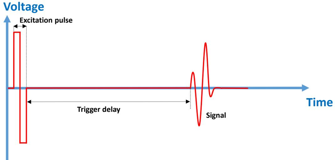
Figure 8 Demonstrate the schematic of an ultrasound signal from the excitation stage to receiving signal stage
