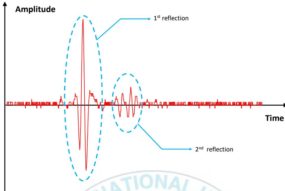
Figure 11 Demonstrate a ultrasonic signal of two reflection
