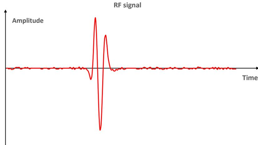
Figure 6 Waveform of a reflective acoustic signal
