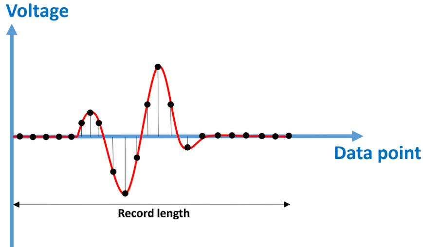
Figure 9 Demonstrate a segment of the signal in digital form
