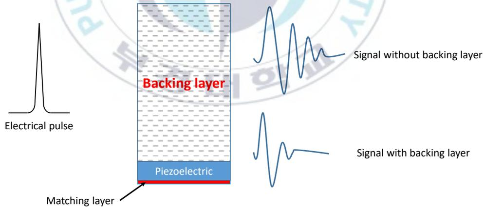
Figure 2 Demonstration of the effect of backing layer
