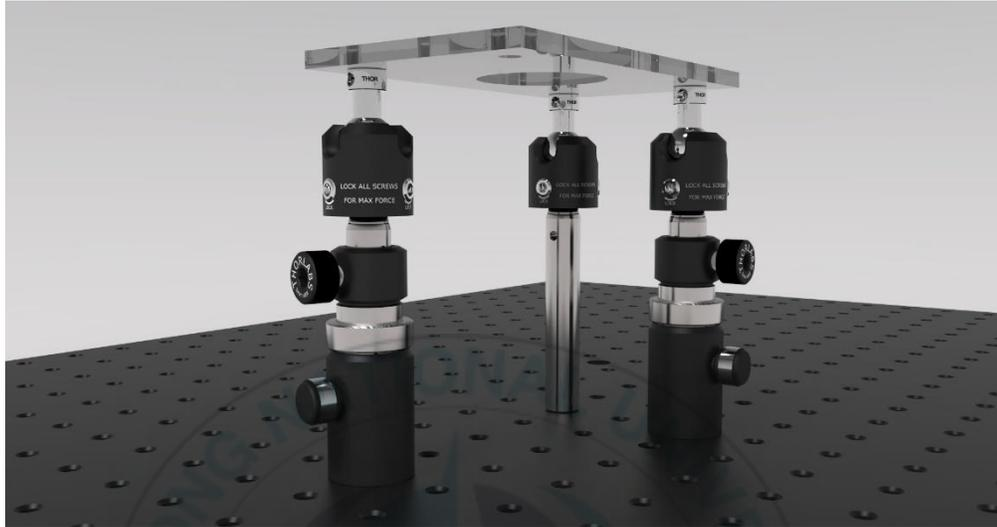
Figure 25 demonstrate tilting adjustable stage
