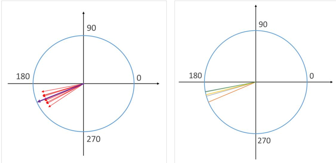
Figure 33 Demonstrate reduction of phase noise effect after average.
