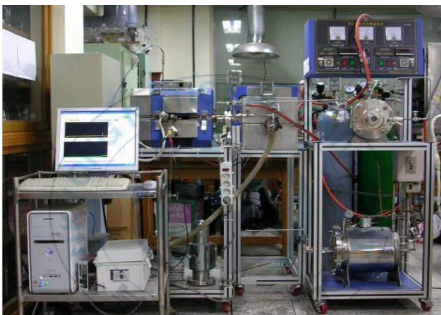
Photo 1. The picture of experimental apparatus for vapor explosion tester.
