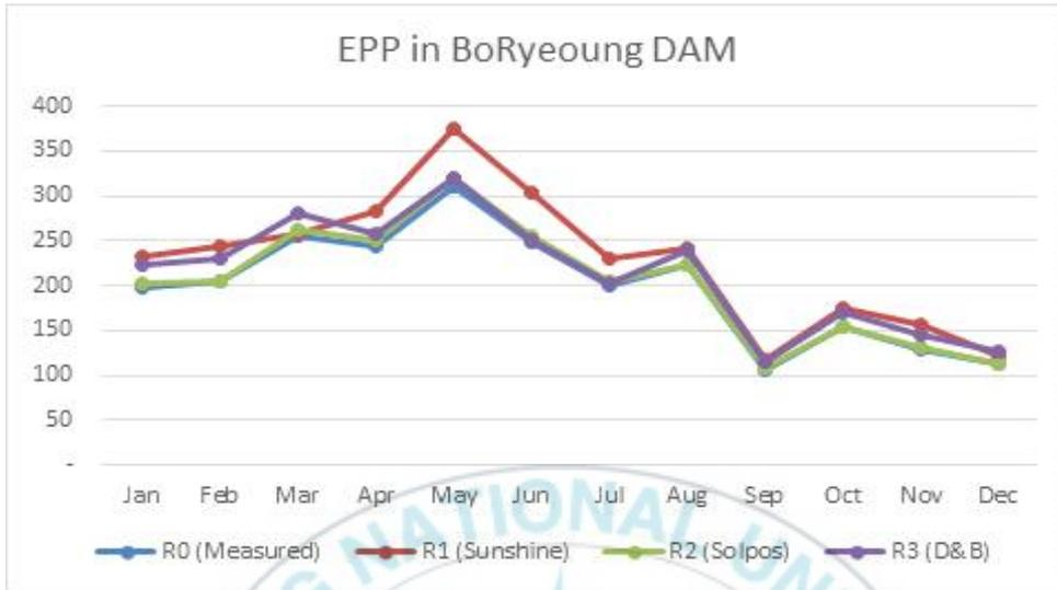
[Figure 5-1] Comparison of Monthly Average PV System Power Generation in Boryeong Dam (unit: MWh)
