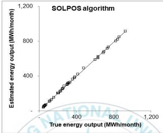
[Figure 5-5] EPP Error Analysis by Solpos Algorithm Method
