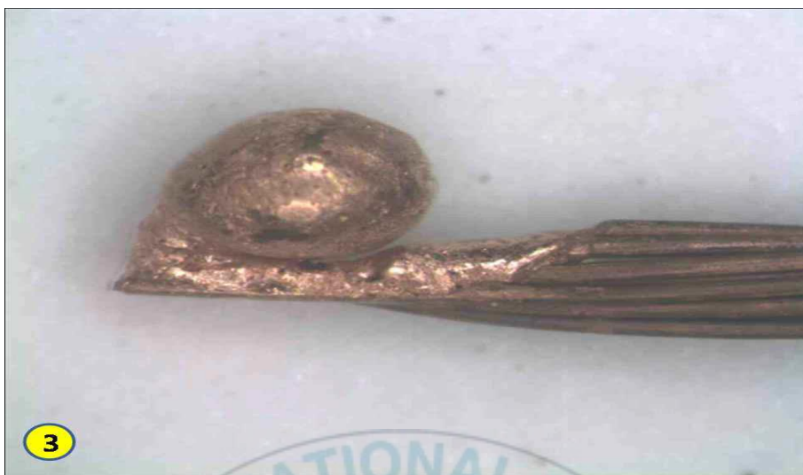
Photo 19. No. 3 stereo microscope on the load side of the water purifier power line(x20).
