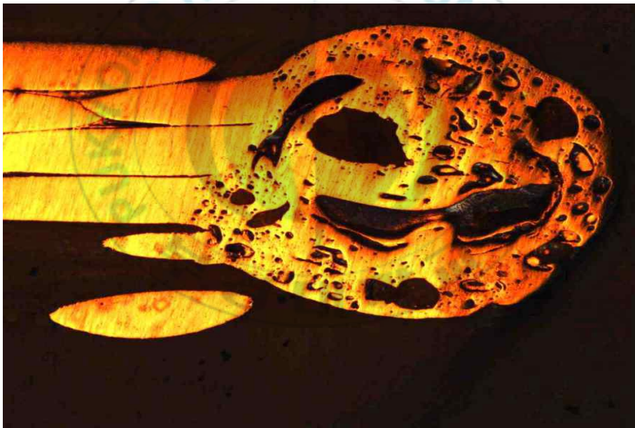
Photo 12. Temperature controller power line(power side) 3-① void (x50).
