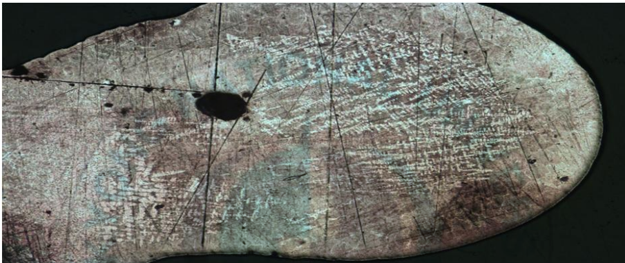
Photo 28. Metal structure of the solid wire melted by heat( \times 50 ).
