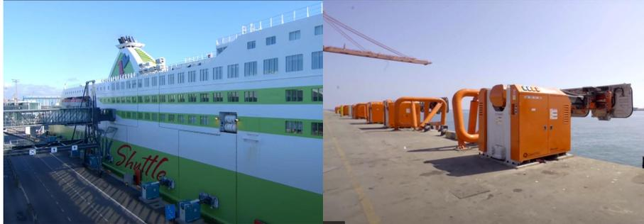
Fig. 1-2 Ship autonomous berthing system(CAVOTEC)
