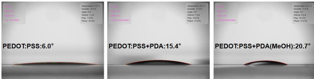
**Figure 9.** Contact angles of water dropped on different PEDOT:PSS films.
