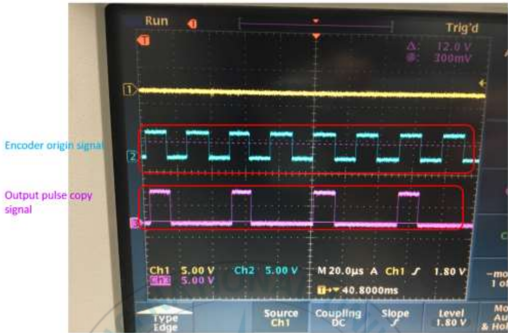
Figure 41: Demonstrate output pulse trigger divide by 2
