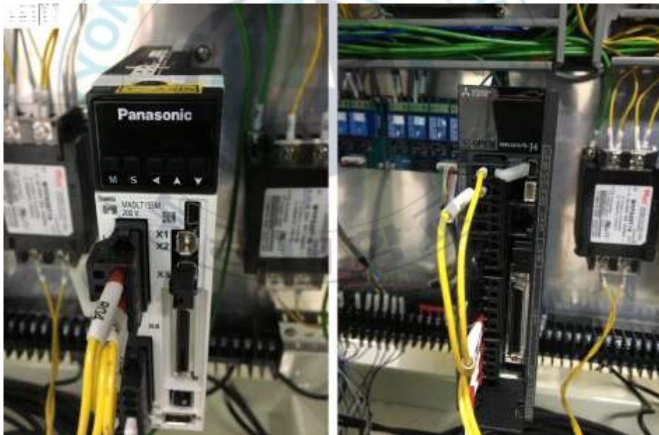
Figure 4: Panasonic MINAS A6 and Mitsubishi MR-J4 servo driver
