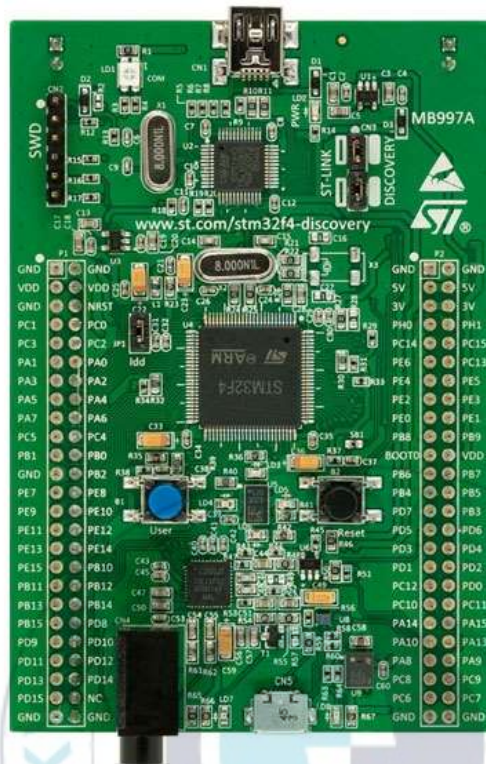
Figure 17: STM32F407VGT6 discovery board [8]
