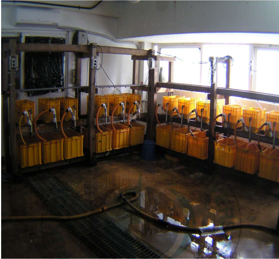
Fig. 7. Photograph of experiment of independent water supply system. Each replication separately re-circulated its water supply in each treatment as shown in the diagram of the experiment layout in Fig. 6.
