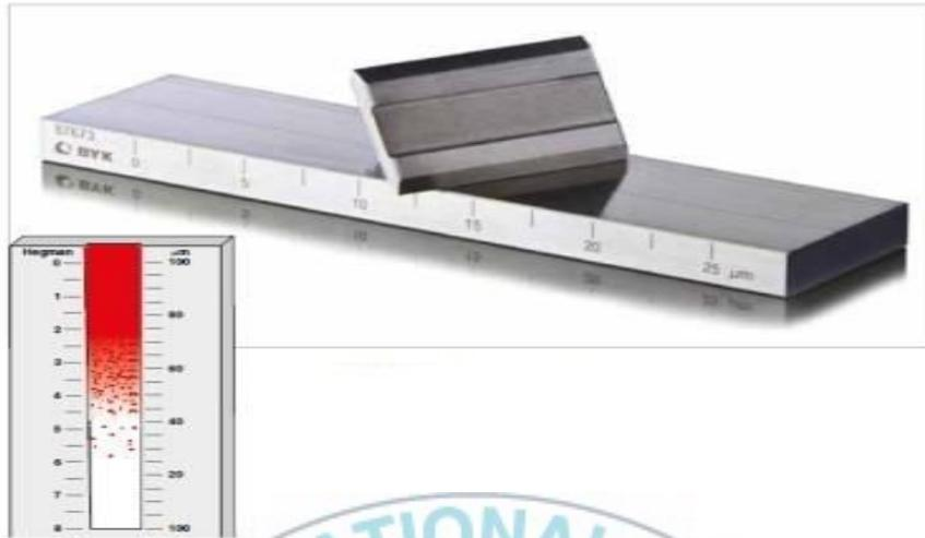
Fig. 18. Image of Grindometer.
