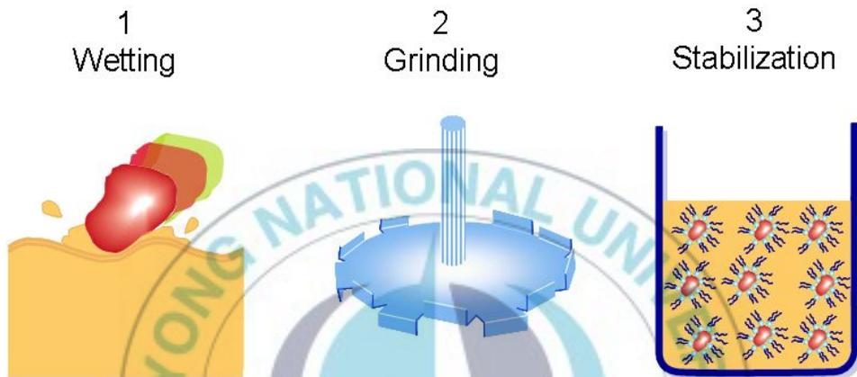
Fig. 10. Three Step of Dispersion Process.
