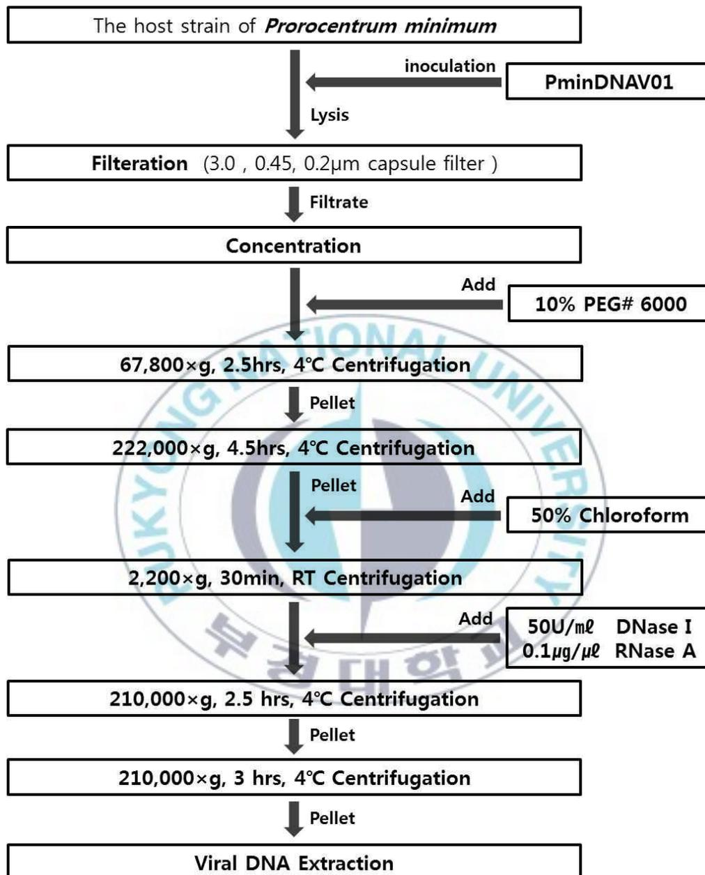
Figure 1. Summarized scheme of algal virus concentration and purification procedure
