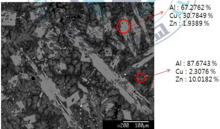
**Fig. 3.55** The result of spot analysis method of uncoated Al - Cu
