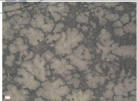
**Fig. 3.20** Microstructure of ZA-3 ;
