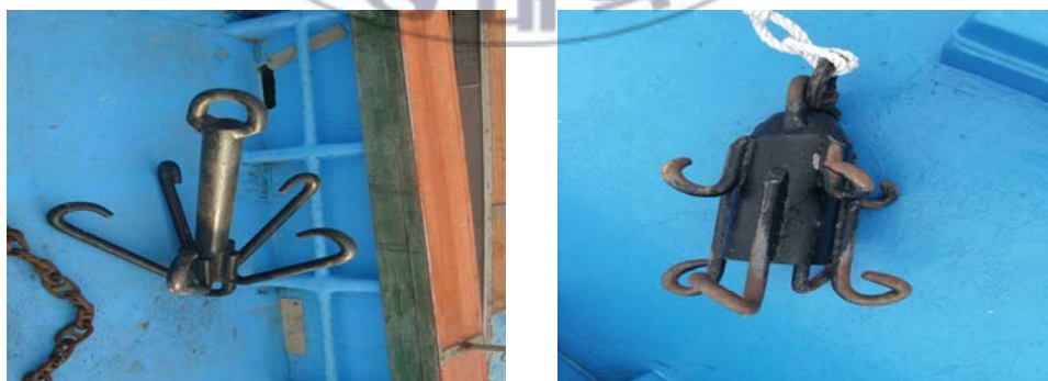
Fig. 9. Type of towing hook for sand, mud(left) and rock(right).
