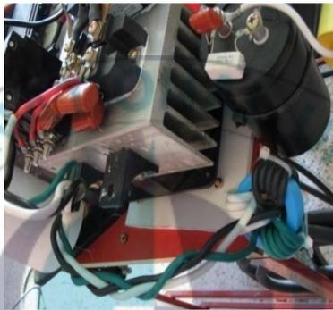
Fig. 2.12 Low frequency rectifier
