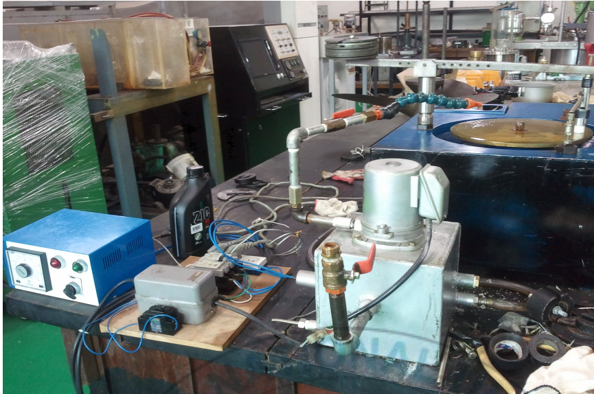
Photo 5. Photos of the pin on the disk wear apparatus
