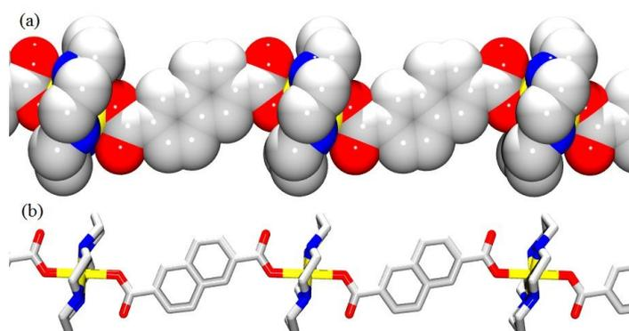
**Figure 1.2.** Space filling diagram (a) and one dimensional coordination polymer chain (b) of  $[\text{Zn}(\text{L})(2,6\text{-ndc})]_n$  (**1**). Hydrogen atoms other than those participating in hydrogen bonds are omitted for clarity.
