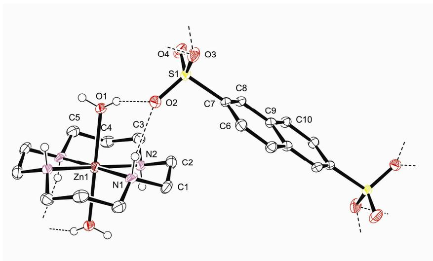
**Figure 1.4.** Molecular structure of  $\{[\text{Zn}(\text{L})(\text{H}_2\text{O})_2](2,6\text{-nds})\}_n$  (**2**) with atom labeling scheme. Hydrogen atoms other than those participating in hydrogen bonds are omitted for clarity.
