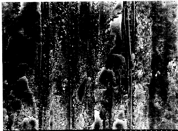
Fig.18 Micrographs of the worn surface of the composite tested on a pin-on-disc device against lay-up orientation [0/90]_{12s} at P=24N , v=1.3m/s .
