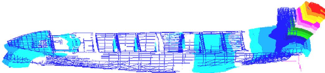
(a) Longitudinal mode of deckhouse coupled with hull girder mode and double bottom (4.59 Hz)
