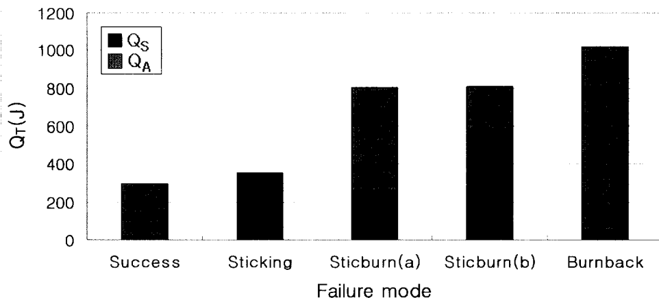
Fig. 4.6 Q_S AND Q_A according to failure mode
