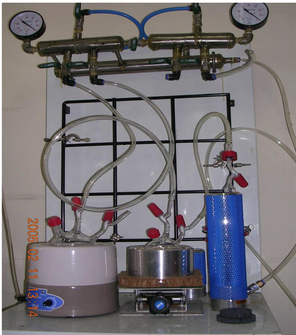
**Fig. 3. Monomer purification equipment.**
