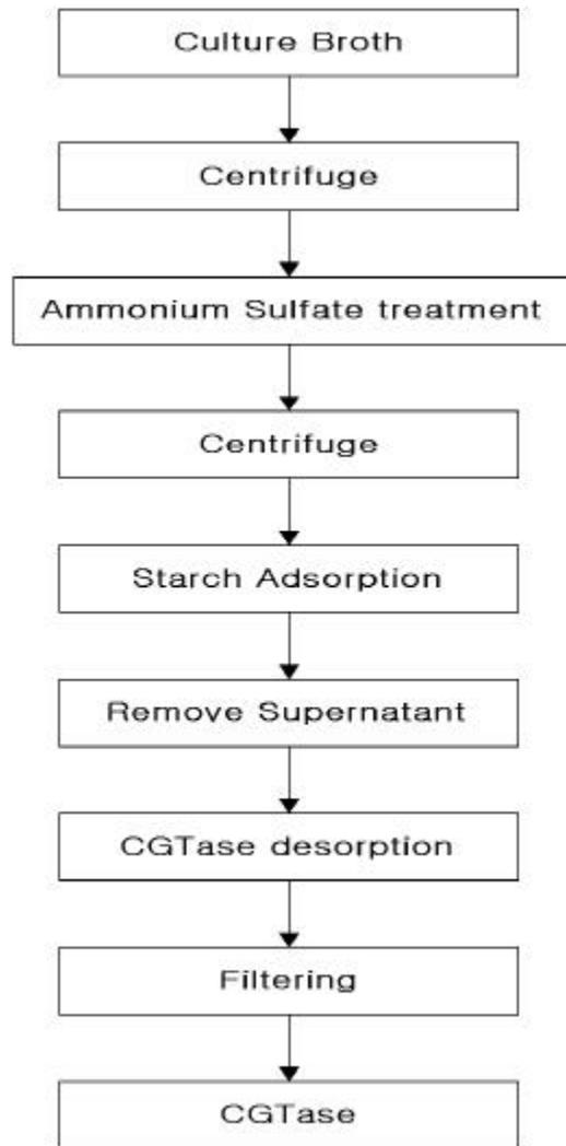
*Figure 1.* The protocol of starch adsorption and desorption
