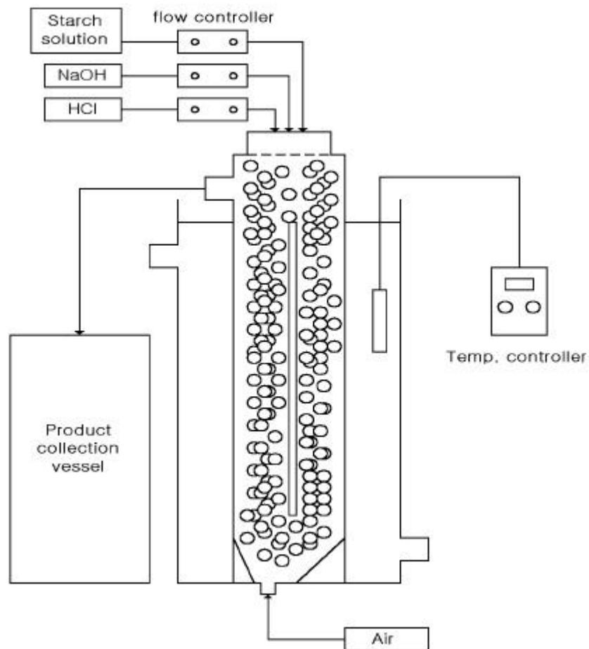
*Figure 2.* Fluidized bed reactor using immobilized CGTase
