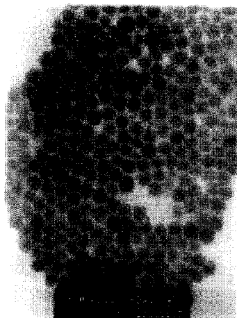
Fig. 2-4 TEM image of nanosized-SiO 2 nanoparticles
