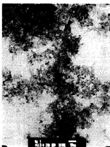
Fig. 2-10 TEM image of CaO nanoparticles
