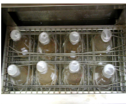
(c) Shaking at thermohydrostat
