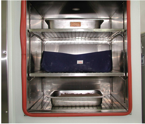
(a) Dried contaminated and un-contaminated soil at 35°C
