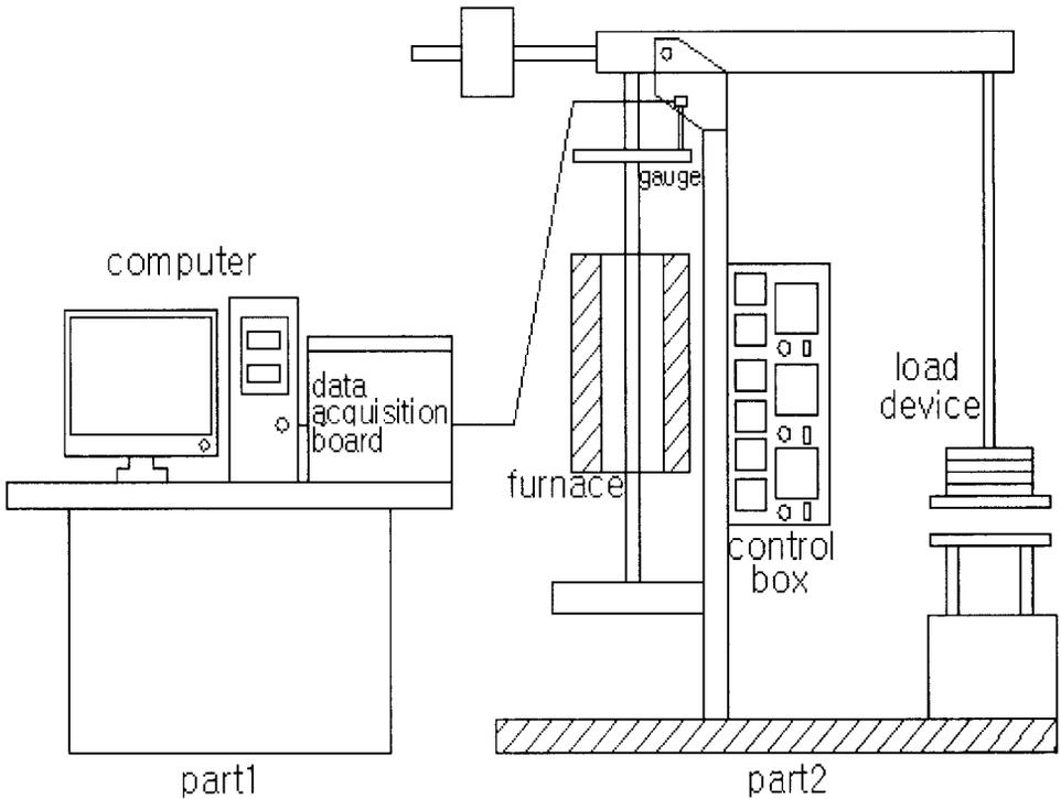
Fig.3 Equipment for creep test units
