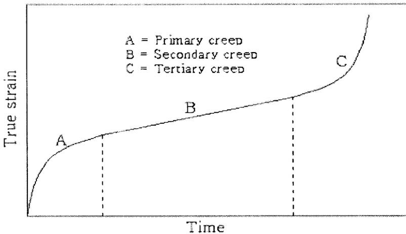
Fig.1 Typical creep curve
