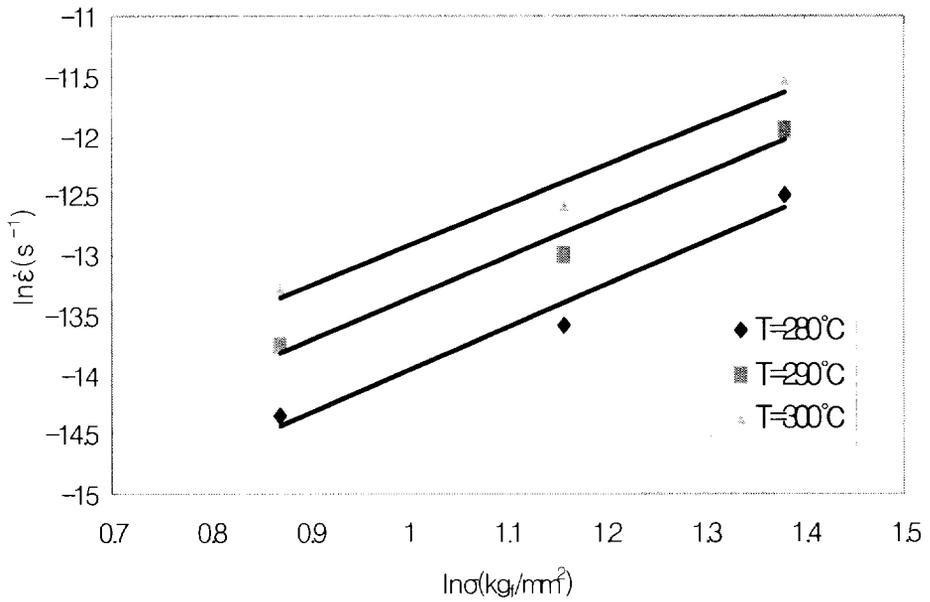
Fig.15 Stress-dependent of creep rate under 280~300°C
