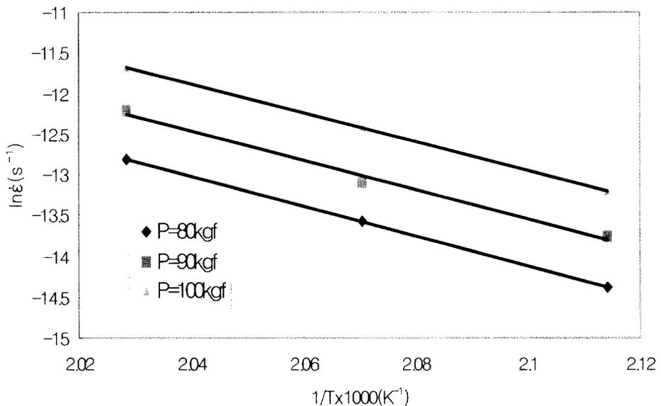
Fig.11 Creep rate vs. the inverse of temperature at load of  $80\sim 100\text{kgf}$
