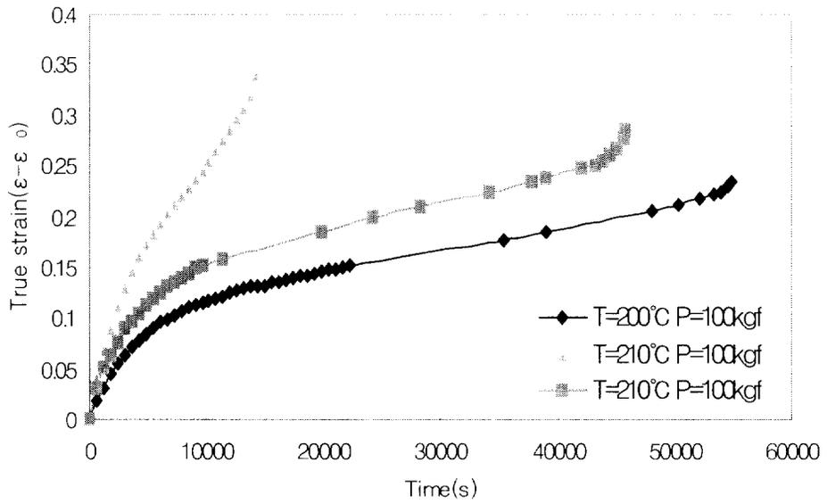
Fig.7 Family of creep curves at 100kg<sub>f</sub>
