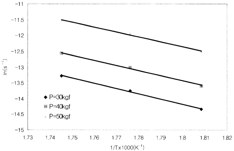
Fig.12 Creep rate vs. the inverse of temperature
