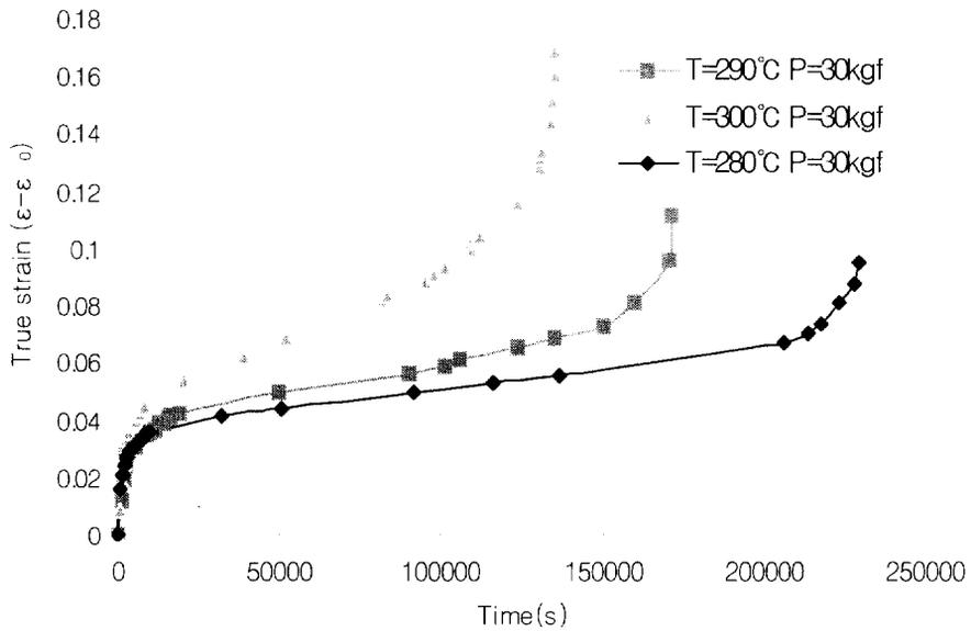
Fig.8 Family of creep curves at 30kg<sub>f</sub>
