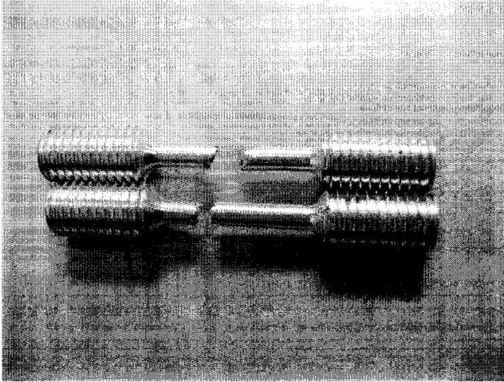
Photo.6 Specimens at the rupture of creep
