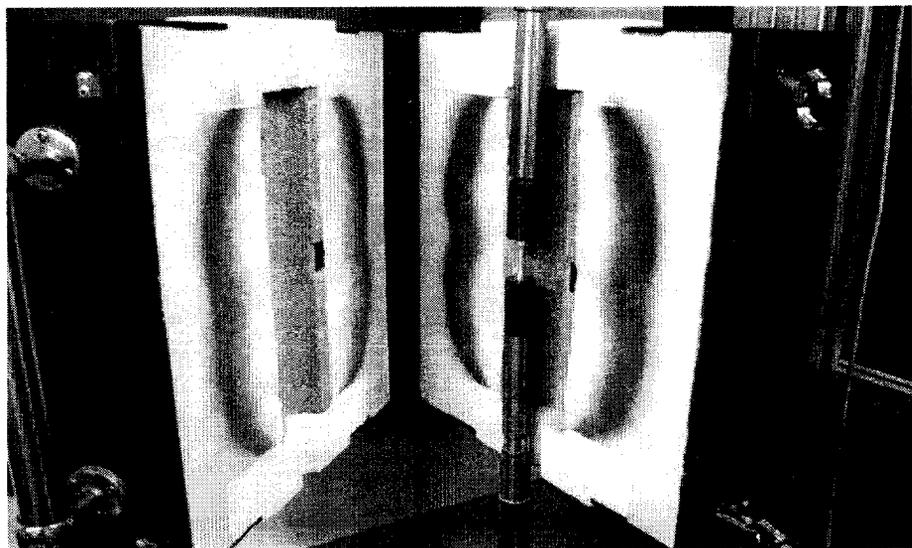
Photo.5 Creep specimen of inner furnace
