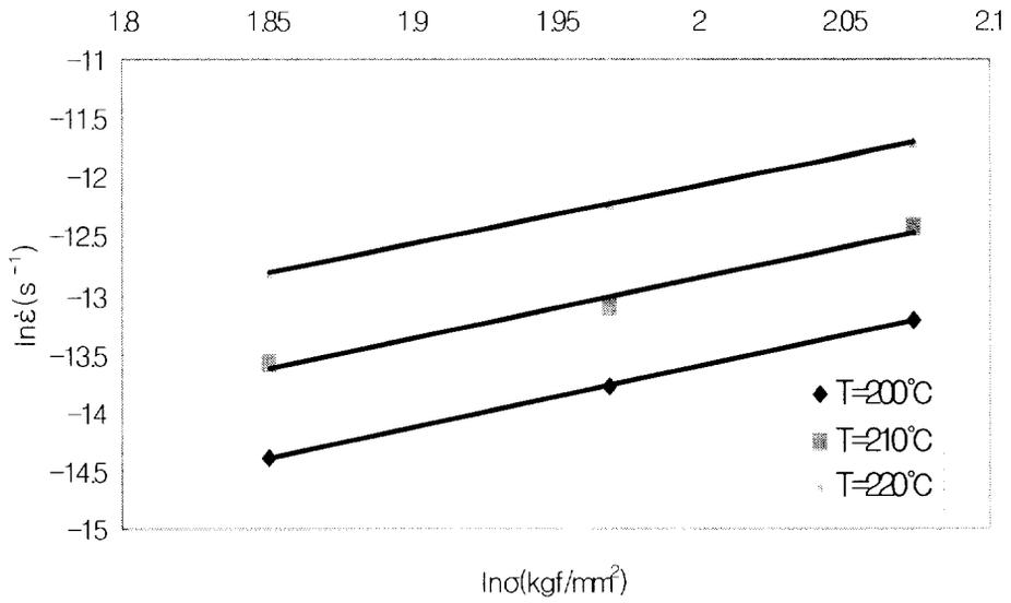
Fig.14 Stress-dependent of creep rate under 200~220°C
