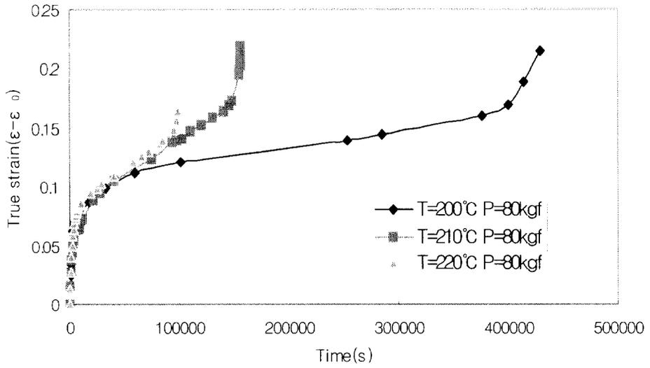
Fig.5 Family of creep curves at 80kg<sub>f</sub>
