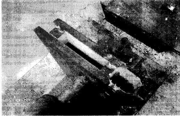
Photo.2 Mold for ZM31 magnesium alloy
