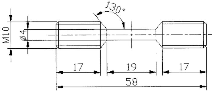
Fig.2 Creep specimen
