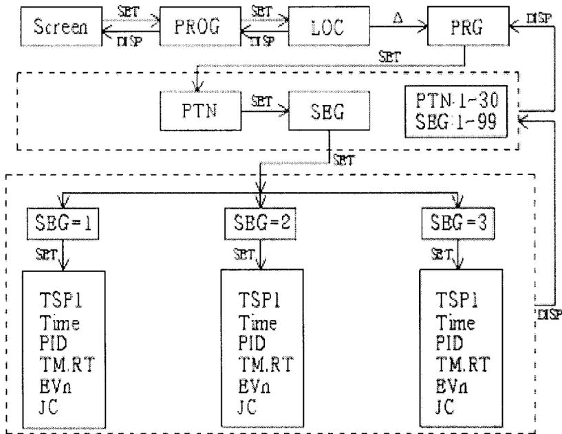
Fig.4 Flow chart for setting of temperature
