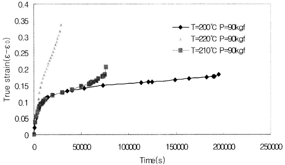
Fig.6 Family of creep curves at 90kg<sub>f</sub>
