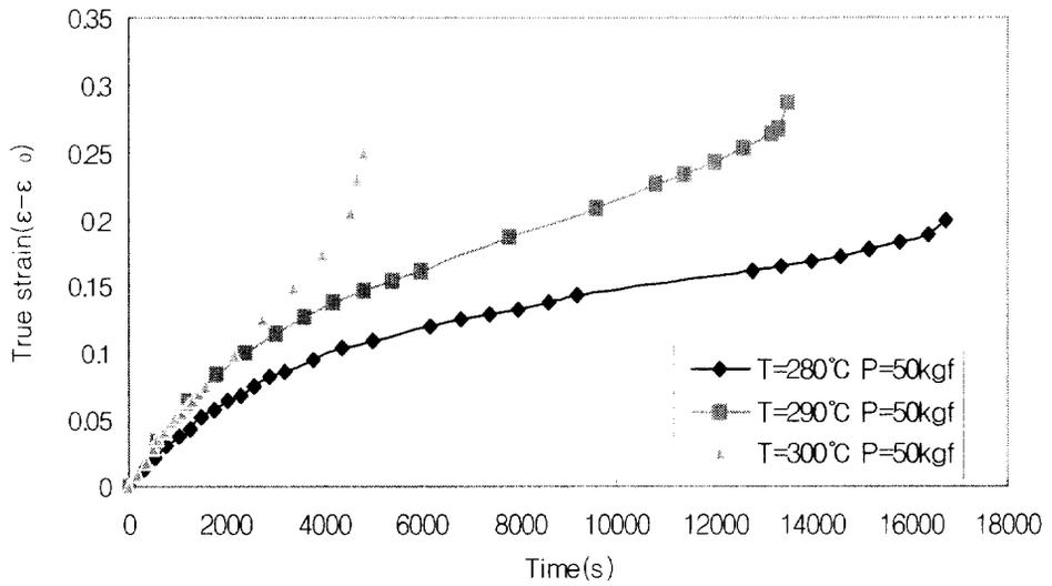
Fig.10 Family of creep curves at 50kg<sub>f</sub>
