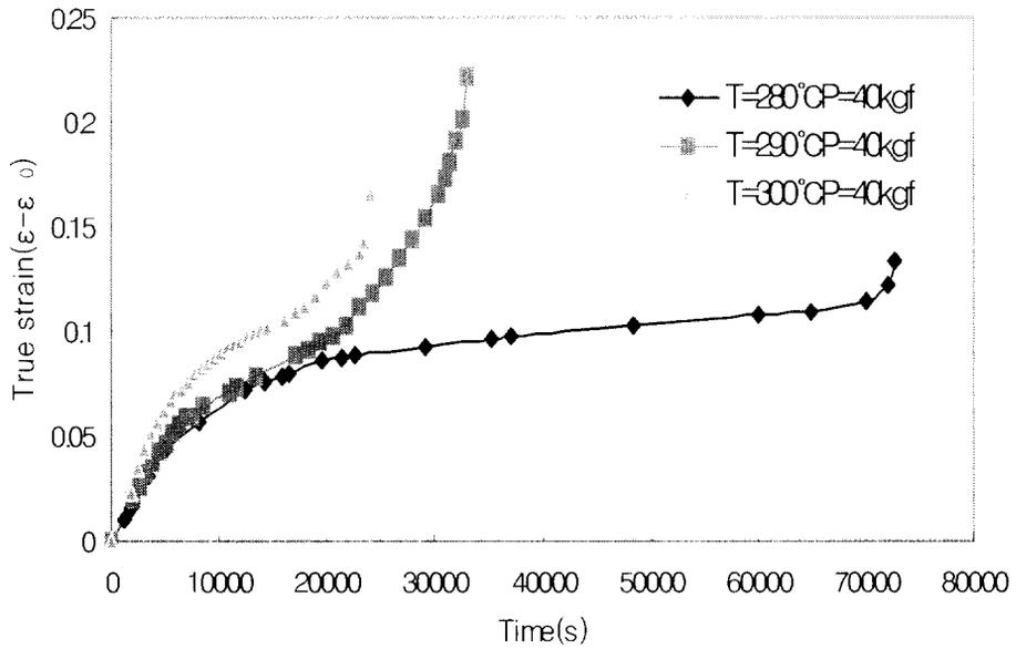
Fig.9 Family of creep curves at 40kg<sub>f</sub>
