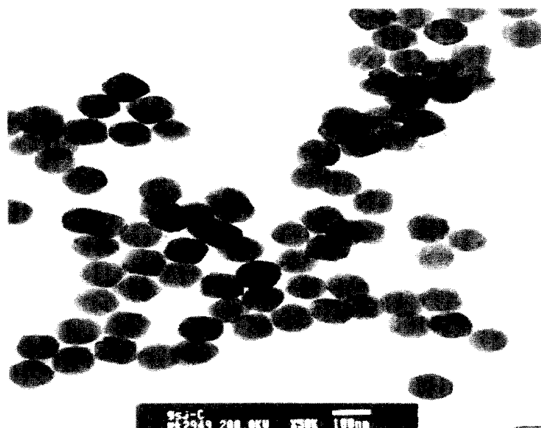
Fig. 18. Transmission electron micrographs(TEM) of hematite particles obtained with cation surfactant MICONIUM DSDM75 (1.0g/L) at 0.02M \text{FeCl}_3 and 100°C, 12h.
