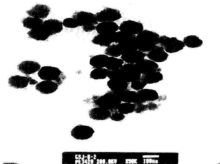
Fig. 14. Transmission electron micrographs(TEM) of hematite particles obtained with amphoteric surfactant MITAIN CA (0.5g/L) at 0.02M \text{FeCl}_3 and 100°C, 12h.
