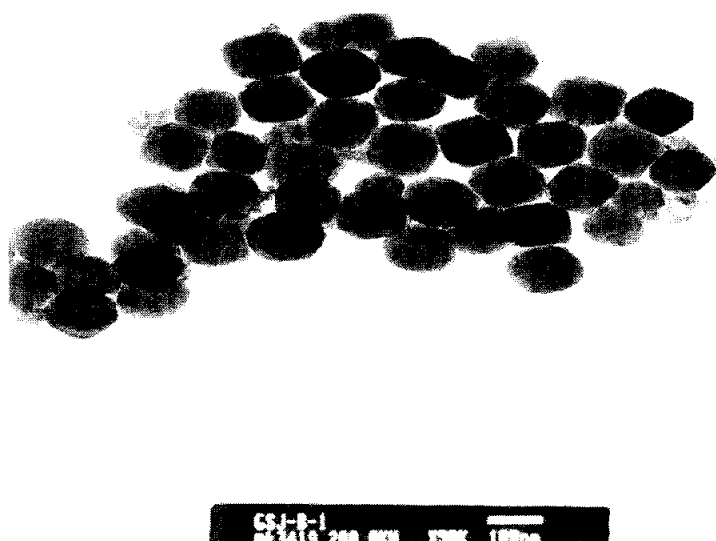
Fig. 13. Transmission electron micrographs(TEM) of hematite particles obtained with amphoteric surfactant MITAIN CA (0.1g/L) at 0.02M \text{FeCl}_3 and 100°C, 12h.
