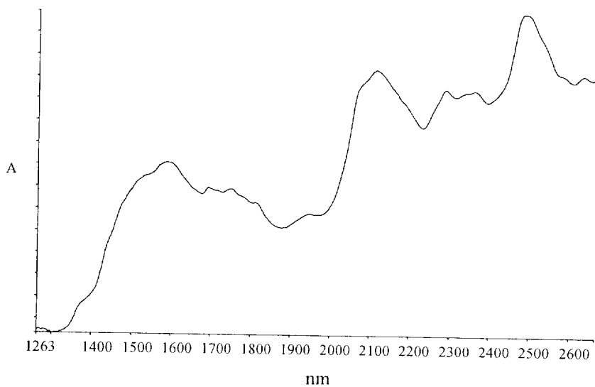
Fig. 20. Near infrared(NIR) spectrum of sorbitol added in surimi.
