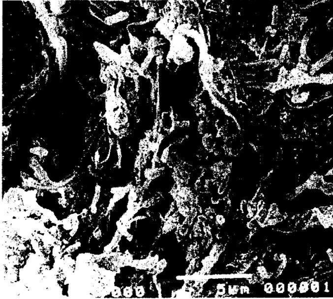
Fig. 4-5. Scanning electron micrograph of bacteria attached on particles of BAC. The carbon particles were taken from upper part of coal-based BAC reactor.
