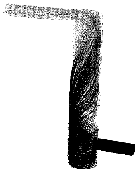
Fig. 4.14 Particle ( 1\ \mu\text{m} ) tracks at the STT (Applied voltage : 0 kV)
