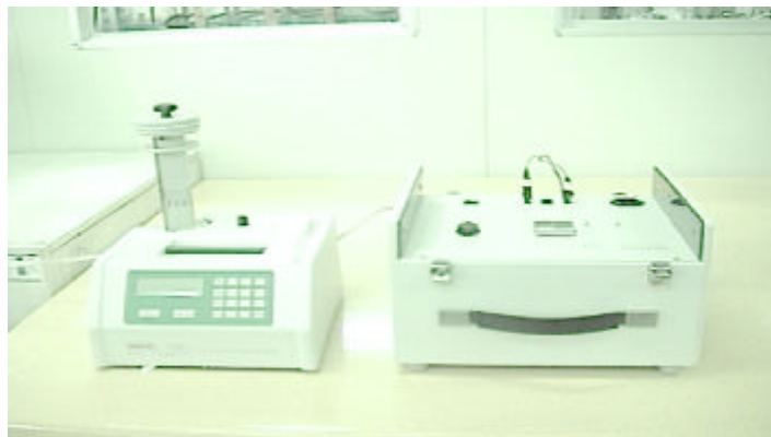
Fig. 2. GS1 gas sampler (GERSTEL Co., Germany)
