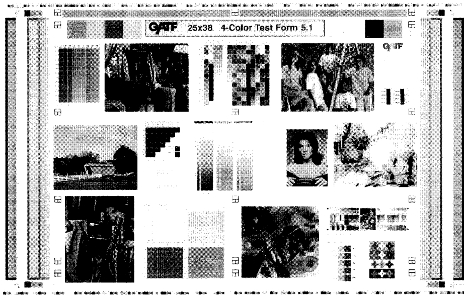
Fig. 3. GATF test form (GATF sheetfed 25X38 inch, 4color).
