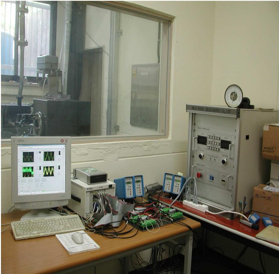
Photo 3.2 Photograph of PXI and dynamometer controller
